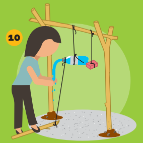
10 Press the stick down with your foot to make the water pour out of the bottle. Put the gravel on the ground below the bottle so that the water soaks away
